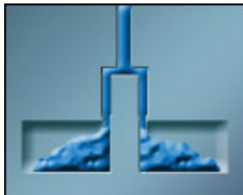
Figure 2: Gravity effect in thick-walled parts
