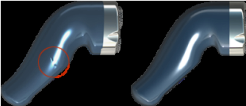
Figure 1: Showcase rendering of digital simulation predicting sink marks and again following design optimization.
