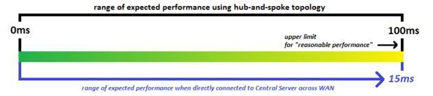
Many firms employ hardware-based data compression technology to reduce traffic across the WAN. Thus a comparable series of tests were run using Riverbed Steelhead devices to observe whether their use had any effect on the range of latencies permissible for directly connecting to the Central Server.
