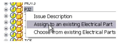
About the AutoCAD Electrical drawing, *PJ2* is the RefDes specified for the connector that connects to the motor MOT2, the motor for horizontal adjustment.
