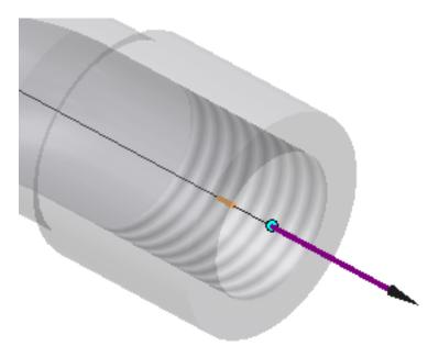
The **Angle** field shows the angle between the two axes. In this example, 88 degrees is used.
