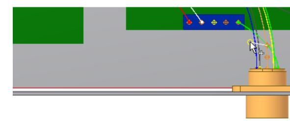
8 Continue selecting points around the printed circuit board (PCB) and toward the other connector to create the segment shape.
