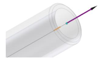
**NOTE** For the Tubes, Pipes, and Hoses part types being authored, you do not have to specify the Pipe Length parameter for connections other than Connection 1. The Pipe Length parameter is unique for a conduit part.
