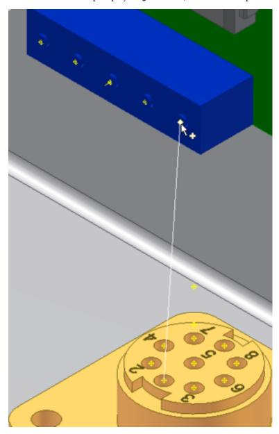
**6** To create the wire, click **Apply**. The wire is created as centerline or rendered, depending on your display setting. By default, the display is set to centerline for wires and cables.
