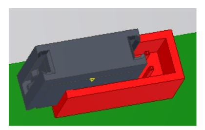
**10** For the final mate constraint, click the right side of the ribbon cable connector.
