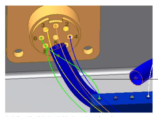
On the Route Wires dialog box, the Wires button changes from red to white to indicate that the wire selection is complete.
