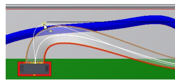
**9** Click in the graphics window to control the approach for the end connector. This time, click an existing work point (2).
