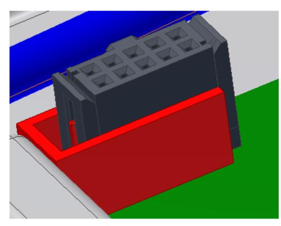
${\bf 7} \quad \text{For the second mate constraint, click the top face of the ribbon cable} \\$ connector.
