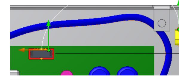
The outward direction on the end connector is not correct. Click the outward direction tool in the End Connector area to change the direction.
