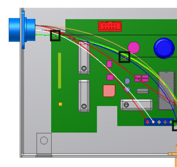
A grounded work point is created at each pick location, and the wire recomputes, changing shape slightly after each point is added.
