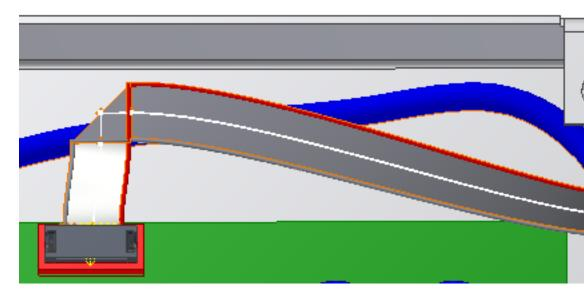
**4** In the browser, expand the Ribbon Cables folder and the ribbon cable. You should see Ribbon1, Fold1, and Ribbon2.
