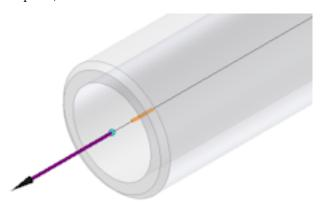
**TIP** If the axis points toward the inside of the part, click **Flip Direction**. The connection direction must point toward the engaging fitting, so it often points outward.
