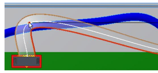
An arrow appears at the fold point indicating the direction of the next work point n the path of the ribbon cable. It is the correct direction for this fold.
