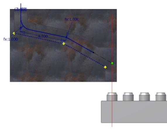
5 After the dashed line and the intersection point appear, click the sloping segment to set the snapped route point.
