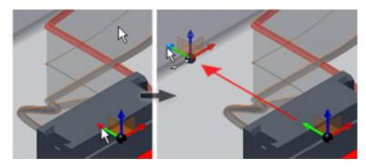
**22** Select the **blue** arrowhead, and drag the triad approximately -0.3 in (negative 0.3 in) from its current location.
