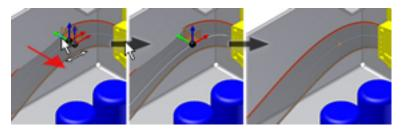
25 You can edit the twist of any intermediate spline point, unless a fold consumes the point. Right-click the spline point, and select **Edit Twist**. Drag the twist arrows.
