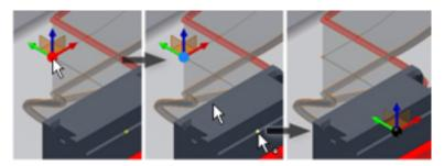
21 Select the **green** arrowhead, and drag the triad approximately 0.9 in along the Y axis. Alternatively, you can click the green arrowhead, and enter 0 . 9 in the  $\mathbf{Y}$  control of the 3D Move/Rotate dialog box.
