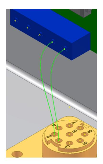
10 Click **Finish Cable and Harness** to exit the Cable and Harness environment. You can view the added wires in the browser when you expand the **Wires** folder under **Harness Assembly1**.
