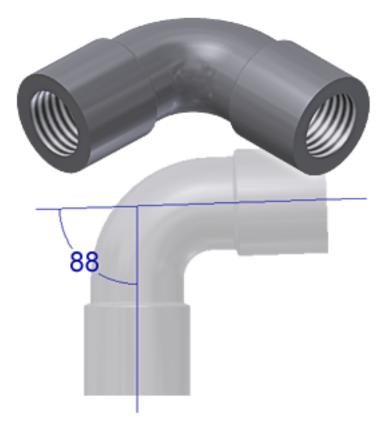
This elbow was created so that there are 88 degrees between connection axes. The elbow is ready for authoring and publishing. No further design work is needed.
