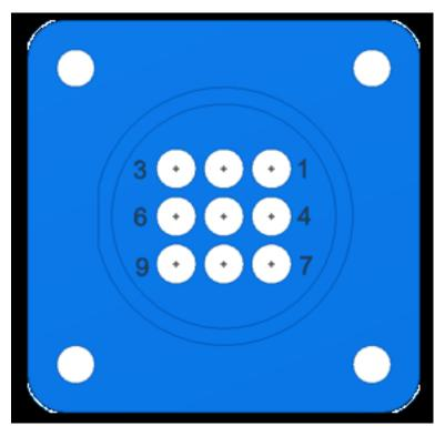
2 In the browser, expand the PCB subassembly to locate and edit part LTP. Add the pins as shown. Pin 1 is the pin closest to part 360124. Assign the RefDes placeholder J?.
