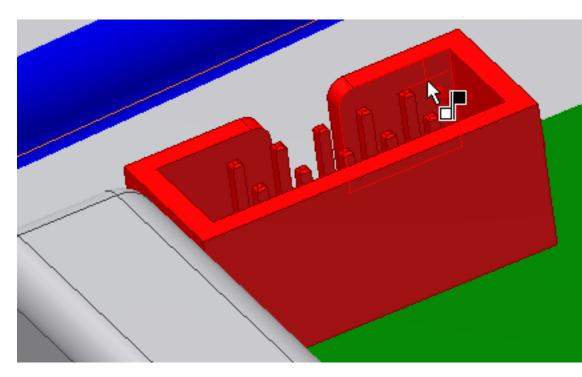
**6** When the preview shows the connector has moved into place, click **Apply** to create the first mate constraint.
