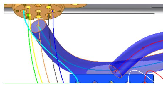
The wire is routed into the main segment and out the branch. The segment diameter and wire length are calculated automatically.
