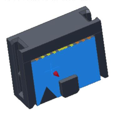
5 The second selection tool is now active. Click the wall of the **RC Male Connector** as the geometry to mate to.
