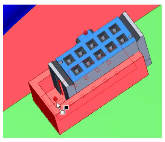
9 When the preview shows the connector has moved into place, click Apply to create the second mate constraint.
