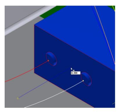
11 Click additional points along the enclosure walls. Ensure that the offset is shown to the interior of the enclosure. If the blue offset line is not visible, the point is created on the exterior of the enclosure.
