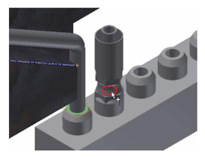
11 Click to place the end fitting. The route line displays.
