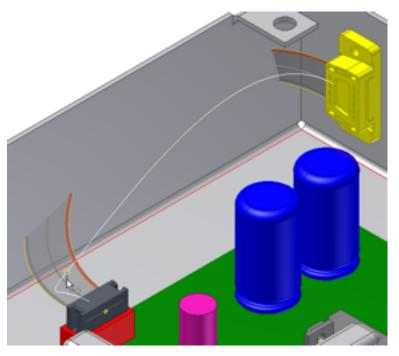
10 Add a point to the spline that is used as a control point to edit the cable twist. Select the housing face, near the end connector, to locate the second point.
