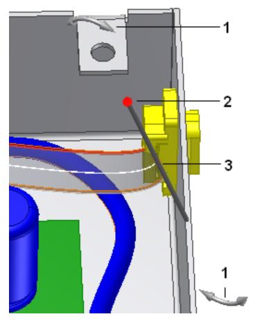
**4** Click and drag a rotation handle until the ribbon body aligns with the slot, and release the mouse button.
