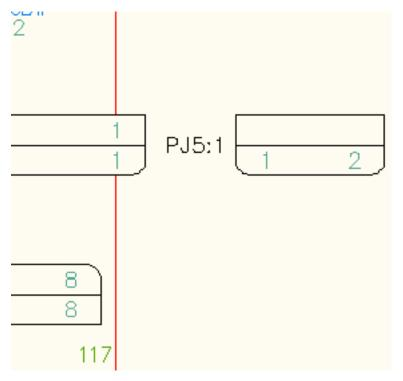
7 In the Connector Selection dialog box click **Wire It**. AutoCAD Electrical connects the pins as you specified in Inventor.
