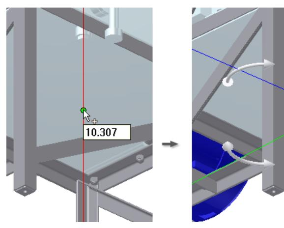
Notice that the green and blue vectors are not at right angles to the red vector. Relative to the red vector, the angle is 88 or 92 degrees, depending on how you measure. The custom fitting you specified in the self-draining style determines this angle.
