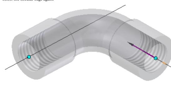
**Flip** the direction of the connection vector so that it points out and away from the elbow. Both connection vectors point out and away from the fitting.
