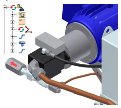
2 The active style is listed in the **Manage** panel of the **Route** tab. Select **Medium Copper Tubing** from the drop-down list.
