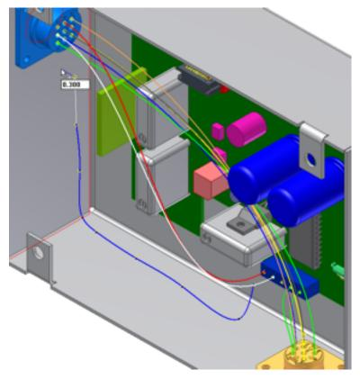
12 With enough points defined, right-click and select **Continue**. The segment is created around the spline points and the **Create Segment** command is still active.
