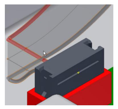
24 In this example, the ribbon cable interferes with the housing around the second intermediate spline point. Use **3D Move/Rotate** to move the point so that the ribbon cable clears the housing.
