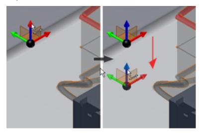
**23** Click **Apply.** The ribbon cable fold adjusts and the 3D Move/Rotate dialog box remains open. If you click **OK**, the fold adjusts and the dialog box closes.
