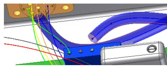
**NOTE** Once a segment is created, you can verify whether any points along the segment violate the bend radius value. In the browser, right-click the segment then select **Bend Radius** ➤ **Check** from the context menu. Verify that the bend radius multiplier is set before checking the points. Select "bend radius, check" in the Help index for more details on bend radius checking.
