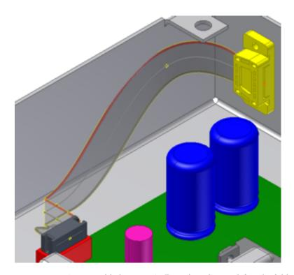
**NOTE** Two points are added automatically to the spline to define the fold geometry fully. The added points are not editable. Their positions are determined automatically as a by-product of the size of the ribbon cable and orientation of the fold.
