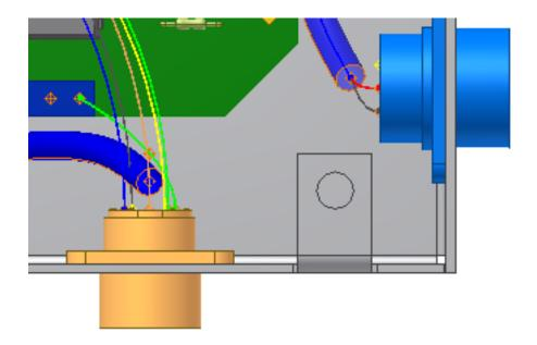
**NOTE** All cable wires are routed or unrouted together and must take the same path (routed through the same segments) in the harness assembly.
