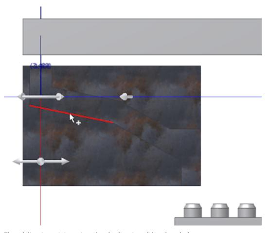
The red direction axis is reoriented to the direction of the selected edge. The included reference geometry is added to the Included Geometry folder in the Model browser.
