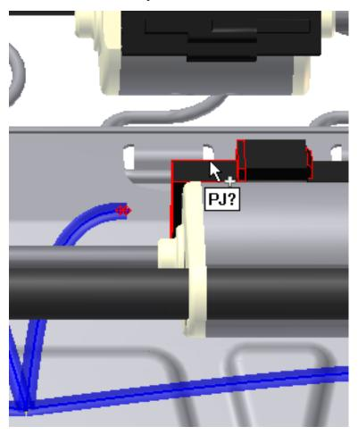
You can select the occurrence in the browser. However, when you use the graphics window, Inventor displays a tooltip. The tooltip shows the RefDes for that component. The Question Mark (?) indicates that the RefDes is not yet assigned.
