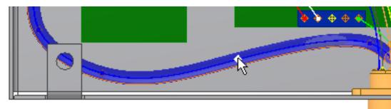
**4** Change the offset to **0.470**, and then select one point (2) between the segment and the LTP:1 connector.
