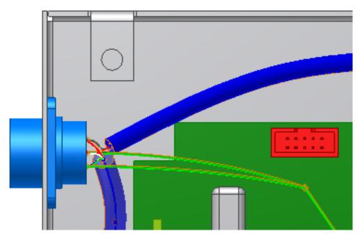
Use **Undo** twice to return the splice to the original location.
