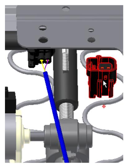
2 On the **Assemble** tab, **Position** panel, use **Grip Snap** or **Move** and **Rotate.** Approximate the position of the connector as shown in the following image. The intent is that the pins on the connector face toward the front of the seat.
