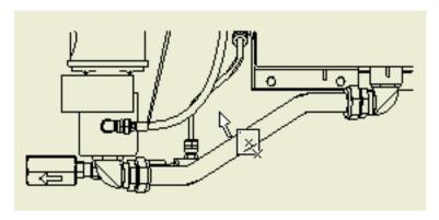
**6** Move the detail view to the desired position, and then click to place the view.
