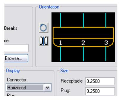
Click **Insert**. Place the connector to the right of the power seat main switch.
