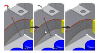
**NOTE** Use the Plus and Minus keys (+ and -) to adjust the size of the twist control.
