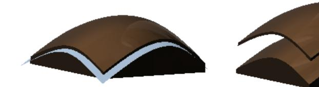
Use Split to divide faces on a surface or solid, or divide a solid into two components. To start, create a work plane, surface, or sketch geometry to use as the splitting tool. Sketch geometry is projected onto the target faces.
