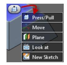
The Selection Tool glyph provides options for selecting geometry and objects.
