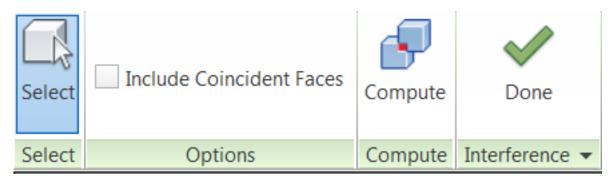
The Interference command analyzes a set of components for interferences. You can select the entire model, multiple components, or a component assembly. Interference does not check for interferences between features within a component.
