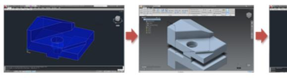
Autodesk Inventor Fusion and AutoCAD both use DWG files. You can use the Open command in Fusion, to open and modify AutoCAD 3D files, and in AutoCAD, to open and modify Fusion files.
