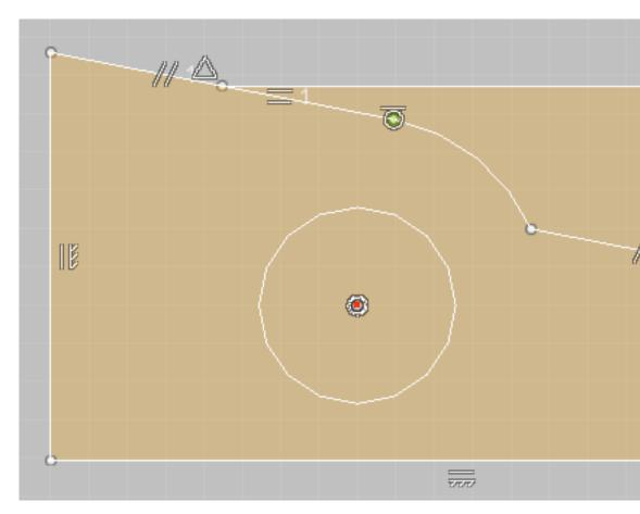
Constraints are automatically created or inferred, while sketching. Constraint symbols dynamically display as you sketch, and the cursor snaps to that position. For example, if a tangent constraint displays while sketching a line, the line preview stays tangent as you move the cursor in that direction.
