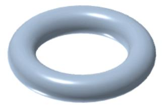
Torus creates a donut shaped Revolve feature by rotating a circle around an axis.
