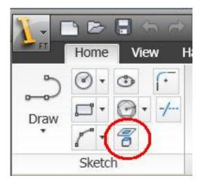
You can project model edges, work geometry, and sketch entities into the active sketch. Projected geometry is locked by default. For more information, see Locking Sketch Geometry (page 124).
