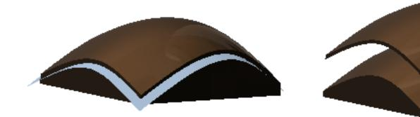
Use Split to divide faces on a surface or solid, or divide a solid into two components. To start, create a work plane, surface, or sketch geometry to use as the splitting tool. Sketch geometry is projected onto the target faces.
